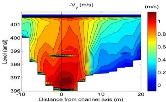
Figure 8: Flow map achieved on the physical model (c.f. Figure 3). Velocity vector field,  $-V_y$ , parallel to the channel axis. Core velocity takes place near the channel axis.
