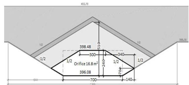
Figure 10: Discharge limiting orifice, with a 9.8 m large, 2.4 m high hexagonal bottom opening of the dam.
