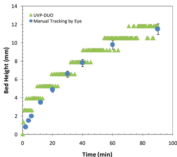
**Figure 3** Tracked sediment bed height over time from the UVP-DUO and from manual measurements
