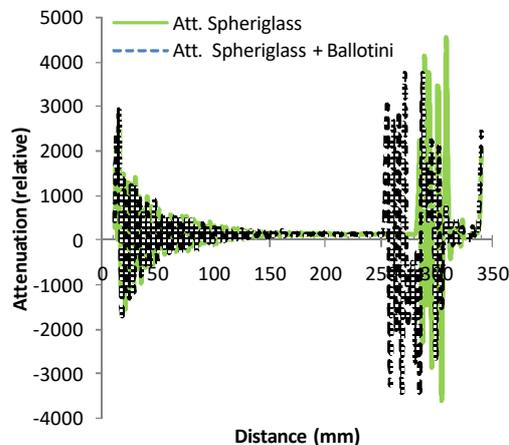
**Figure 4** Average attenuation profiles for a 5 wt% Spheriglass dispersion after 24 hours with and without addition of a Ballotini bed
