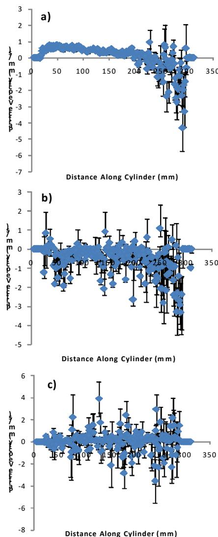
Figure 2 Velocity profile averages for 30 second time steps starting at a) 5, b) 60 and c) 90 minutes
